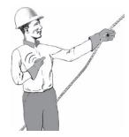
TELESCOPE IN (TELESCOPING BOOMS)
