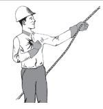
TELESCOPE OUT (TELESCOPING BOOMS)
