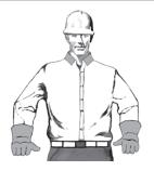
TELESCOPE IN (TELESCOPING BOOMS)
