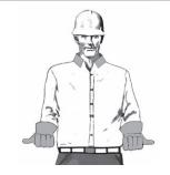
TELESCOPE OUT (TELESCOPING BOOMS)
